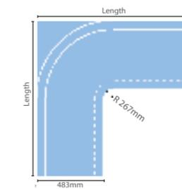
Corner seat profile with 90° radius and uncoated ends. Includes installation kit.
