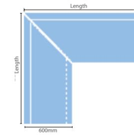
Corner seat profile mitred at 90° with uncoated ends. Includes installation kit.
