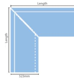
Corner seat profile mitred at 90° with uncoated ends. Includes installation kit.
