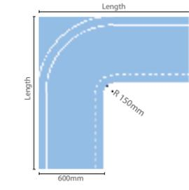
Corner seat profile with 90° radius and uncoated ends. Includes installation kit.
