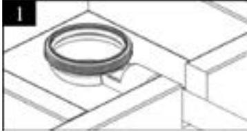
1 Measure Maxxus drain location and then connect section (7) of the gully to the waste pipe using solvent-weld adhesive centrally underneath the hole of the deck.
