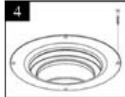
4 Pilot section (4) and screw down using appropriate sized screws. Do not use power tools.
